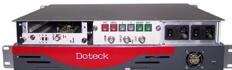
4-slot, 19-inch, dual power supply
