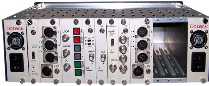
18-slot, 19-inch 3RU, dual power supply
