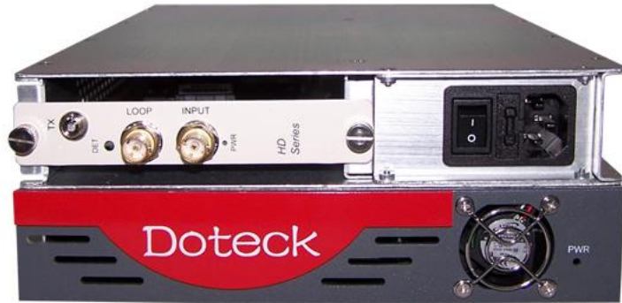
One slot, Built-in power supply
